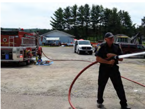
Water from the collapsible reservoir is pumped into the fire truck then out again at high pressure while the tanker, or pumper truck does another run for water at a nearby lake or river.
